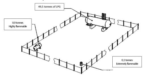
The separation is sufficient that neither small tank can start a major incident at either the other small tank or the large tank.
