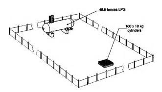
The separation between the compound and the large tank is sufficient to prevent the cylinders starting a major incident at the large tank.
