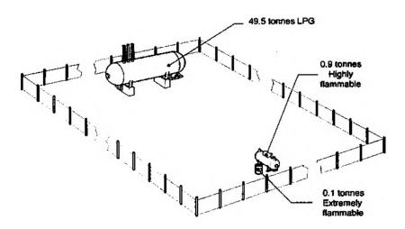
The small tanks are adjacent, but their separation from the large tank is enough to prevent the small tanks starting a major incident at the large tank. The total quantity for application purposes is determined by the aggregation rules, but first it is necessary to determine if the small tanks together exceed 2% of their threshold.
